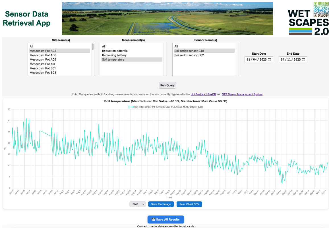
Figure 5: The application's runtime is around 5 seconds for generating a "Soil temperature" plot with data measured with the "Soil redox sensor 048", which is located in the "Mesocosm Pot A03".
